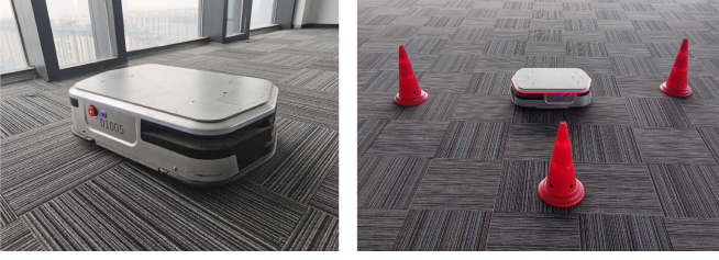
Fig. 4. The UGV and the experiment field. The three red traffic cones serve as landmarks for positioning.
