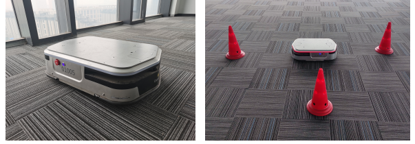
Fig. 4. The UGV and the experiment field. The three red traffic cones serve as landmarks for positioning.
